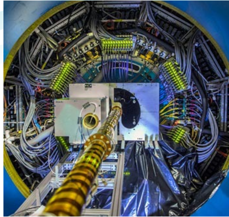
Heavy Flavor Tracker at the center of RHIC's STAR detector. See article on RHIC's 20th anniversary, page 2.
